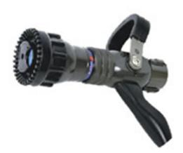
Constant Flow nozzles give constant flow over all discharge patterns, and are lightweight, versatile nozzles, meant to give the operator good control over the discharge. The nozzle gives good range in jet pattern, and a dense fog (due to spinning teeth provided) for radiant heat protection. Can be used for water or foamoperation
